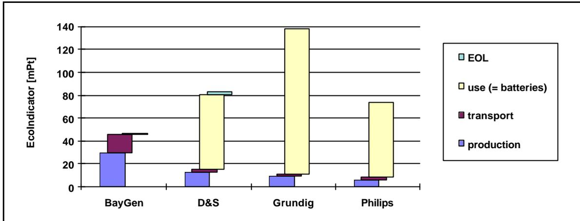
Figure 4 Ecoindicator 95 value for total life cycle of radios
